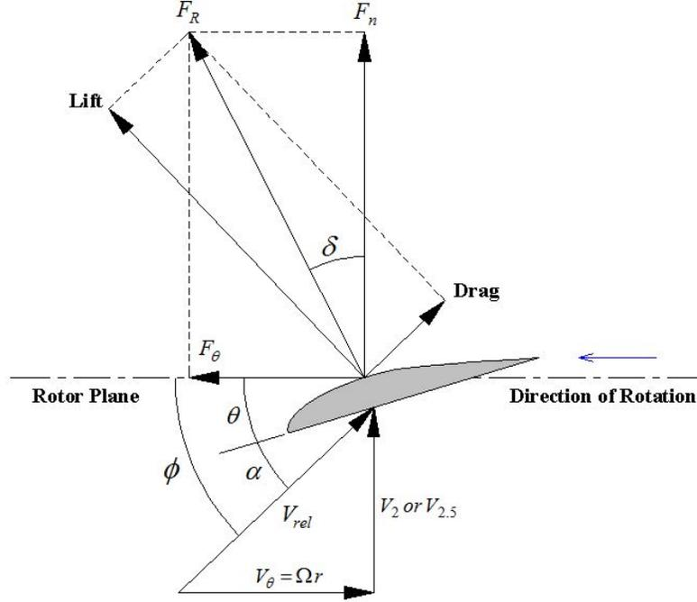
Figure 3. Blade Element, Force and Velocity Triangles
