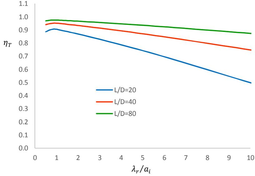
**Figure 4. Annular Blade Element Efficiency**
