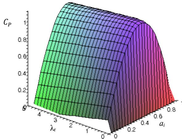
Figure 6.  $C_p$  for Spinner ratio =0.65 and  $L/D=80$
